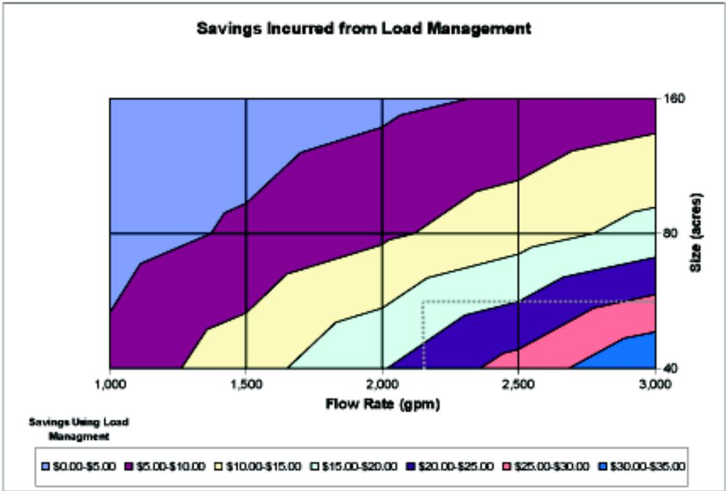
**Fig. 1. The per-acre savings from using load management programs based on field size being irrigated and flow rate. An example is shown where a 60-acre field with a pump making 2,200 GPM will have a savings of \$15 to \$20 per acre by using load management.**
